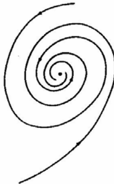
FIG. E, Spiral sink: B = \begin{bmatrix} a & -b \\ b & a \end{bmatrix} , b > 0 > a .
